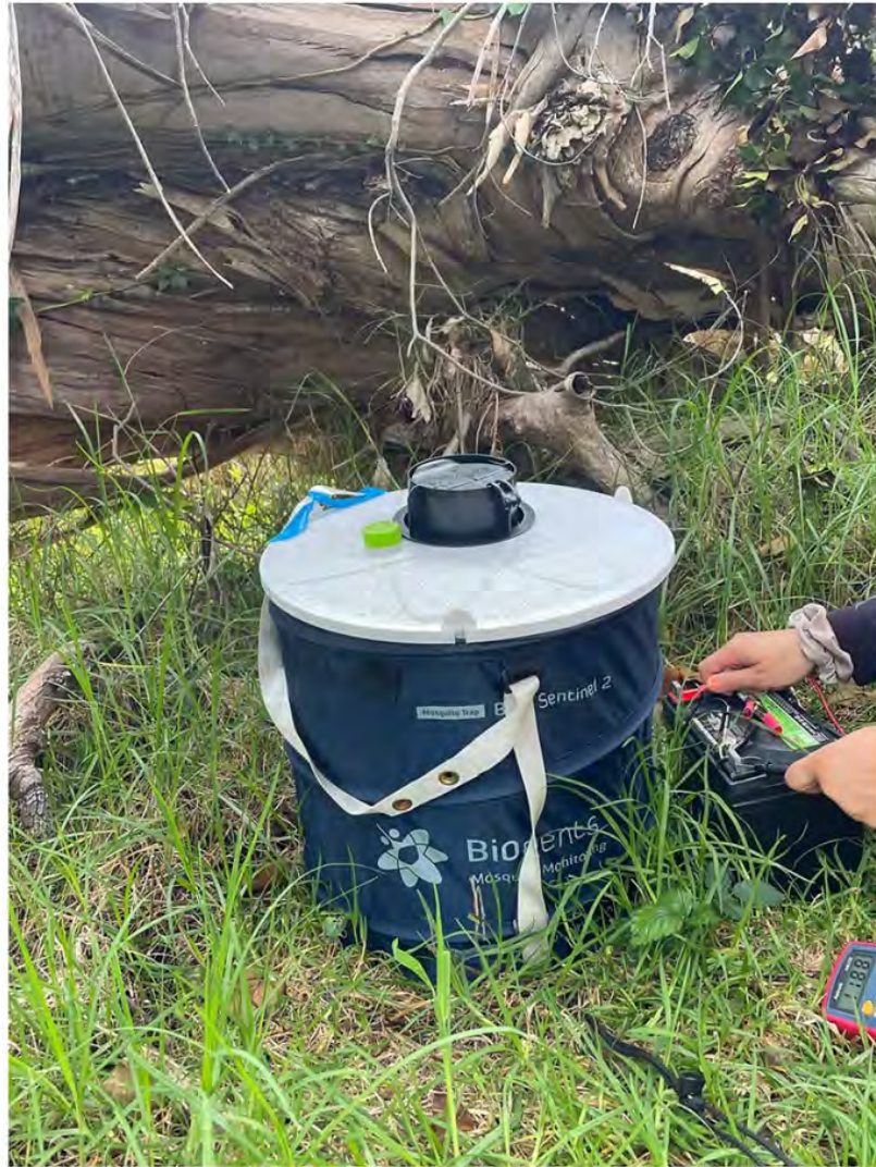
Photograph of a mosquito trap connected to its battery source.
